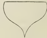
FIG. 2. Section of hull amid ships, old style.
