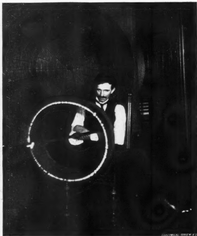
FIG. 7.—"SOME EXPERIMENTS IN TESLA'S LABORATORY WITH CURRENTS OF HIGH POTENTIAL AND HIGH FREQUENCY"—EXPERIMENT SHOWING A COIL ENERGIZED BY THE WAVES OF A DISTANT OSCILLATOR AND ADJUSTED TO THE CAPACITY OF THE BODY OF THE OPERATOR, WHO PRESERVES HIMSELF FROM INJURY BY MAINTAINING A POSITION AT THE NODAL POINT, WHERE THE INTENSE VIBRATION IS LITTLE FELT—THE PRESSURE ON THE END OF THE COIL TOWARDS THE READER, WHICH IS ILLUMINATED BY THE POWERFUL STREAMERS, IS NEARLY HALF A MILLION VOLTS.
